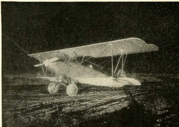
Travelair Plane, painted dark blue, 900 feet from Sperry 18" High Intensity Arc Floodlights at San Francisco Airport.
